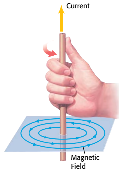
Figure 14-7 Use the right-hand rule to find the direction of the magnetic field around a current-carrying wire.
