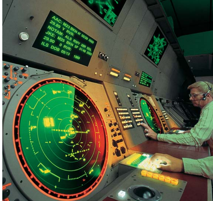
Figure 12-17 The radar system in an air traffic control tower uses reflected radio waves to monitor the location and speed of airplanes.
