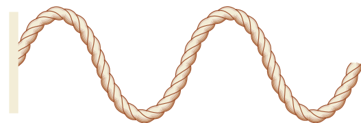
B This transverse wave on a rope is a simple sine wave.
