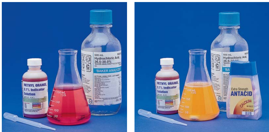
Figure 6-23 Adding antacid tablets to an acidic solution makes the solution less acidic. This is indicated by the color change of the indicator present in the solution.
