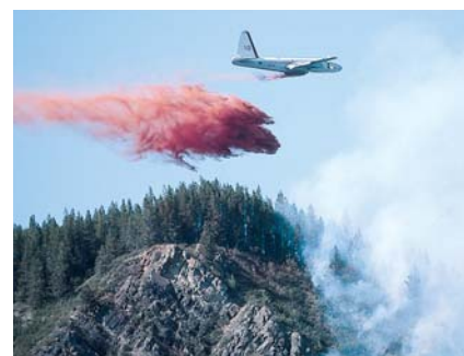
Figure 5-23 Ammonium sulfate and ammonium phosphate are being dropped from the airplane as fire retardants. The red dye used for identification fades away after a few days.
